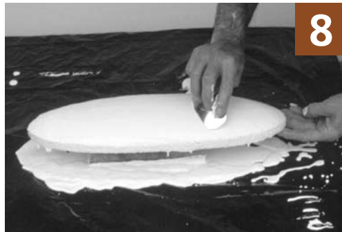
Smooth plaster with metal rib.
