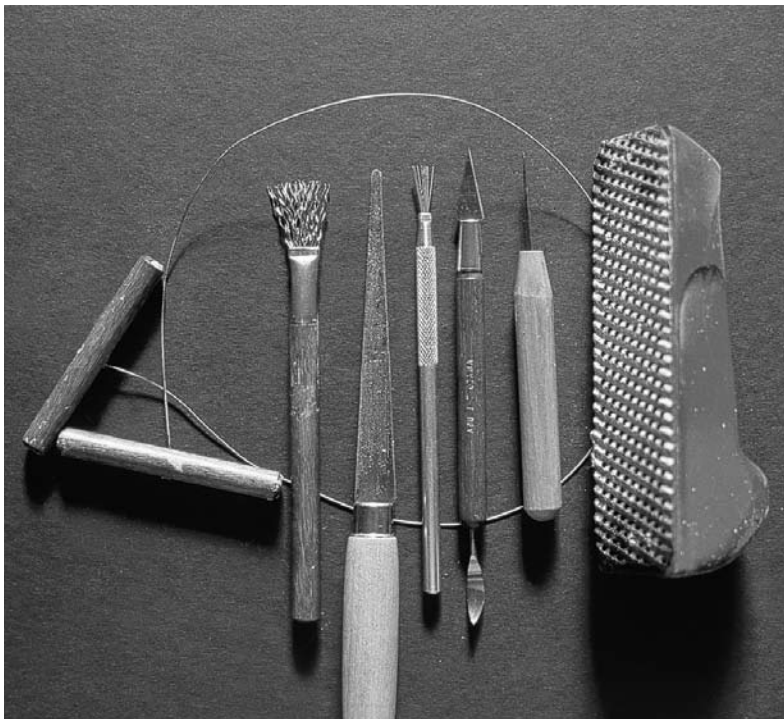
Tools needed include a cutting wire, large scoring tool, fettling knife, small scoring tool, lace tools, needle tool, Surform and brayer or rolling pin (not shown).
