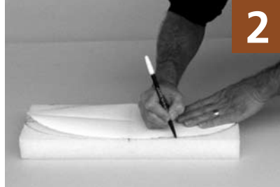
2 Transfer pattern from template.
